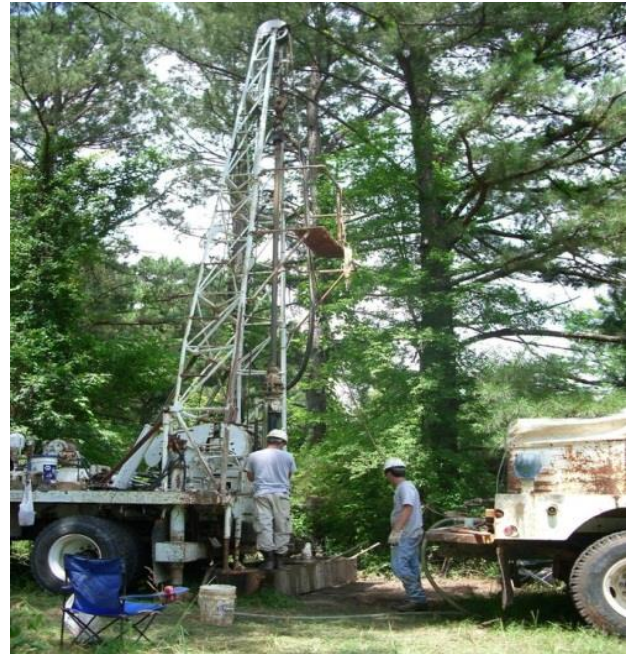
Staff of the Office of Geology drill test holes for geologic mapping and aquifer assessments
